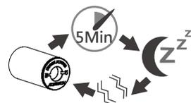
4. Low Battery Force Power off: the indicator LED flashes red, 3 flashes from the flame LED to indicate the battery level is too low and shutdown.
